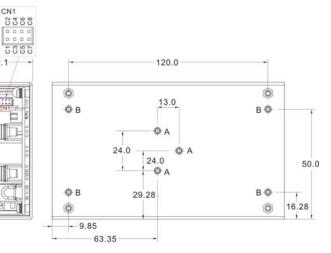
A=For fixture to din rail clip only B=For fixture to pcb/chassis only A=M3x0.5P B=M3x0.5P
