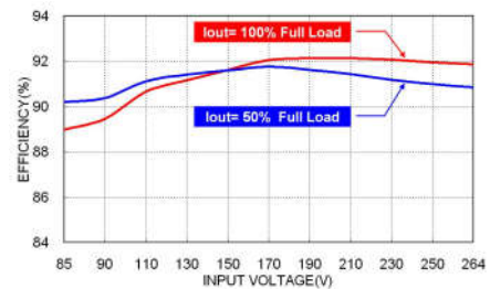
T□D40US24B Efficiency vs. Input Voltage
