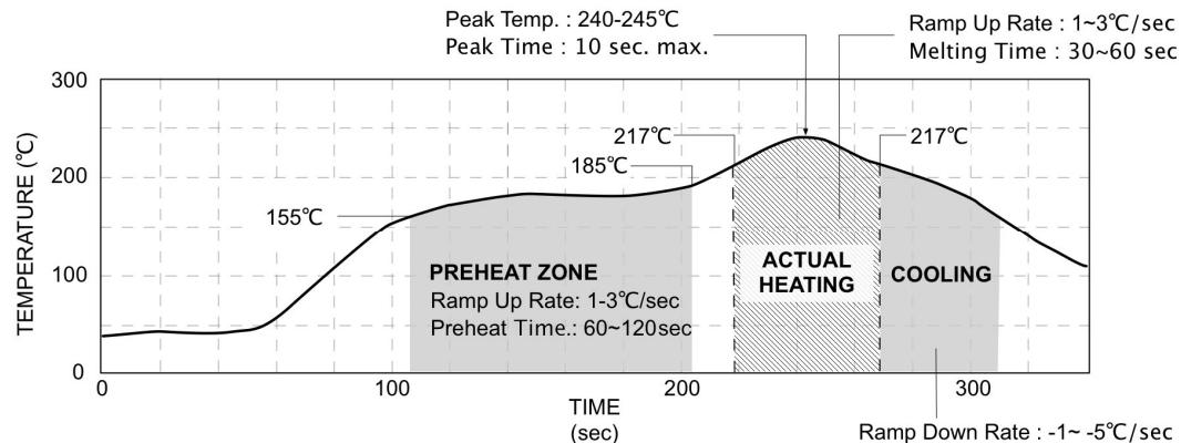
\*The curves define the maximum peak reflow temperature permissible measured on pin1 or Vin pin.
