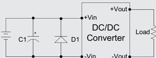
D1: Transient Voltage Suppression Diodes
