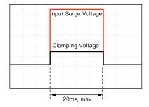
Our surge protector module offers a voltage clamping function to clamp input voltage to a safe value and make the power module keep operating normally.
